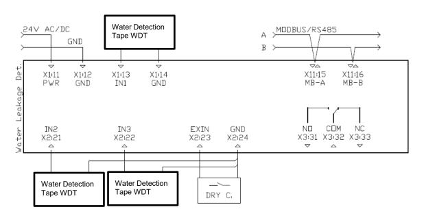
Relay contact rating is max. 1A at 230VAC
